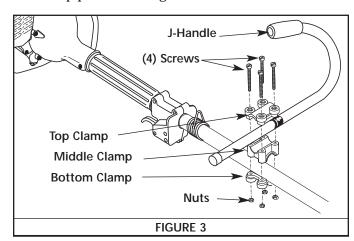
4. While holding the three pieces together, install the four (4) screws through the top clamp and into middle clamp.
